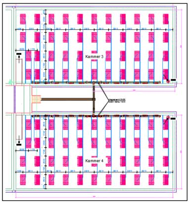
Figure 2: Installation of the MESSNER Aeration Panels
